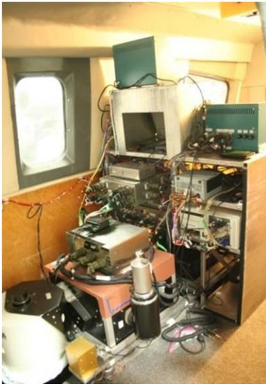
**Figure 4:** View of chemical sensors: high speed infrared spectrometer, lower left corner; infrared line scanner is out of view behind the line scanner
