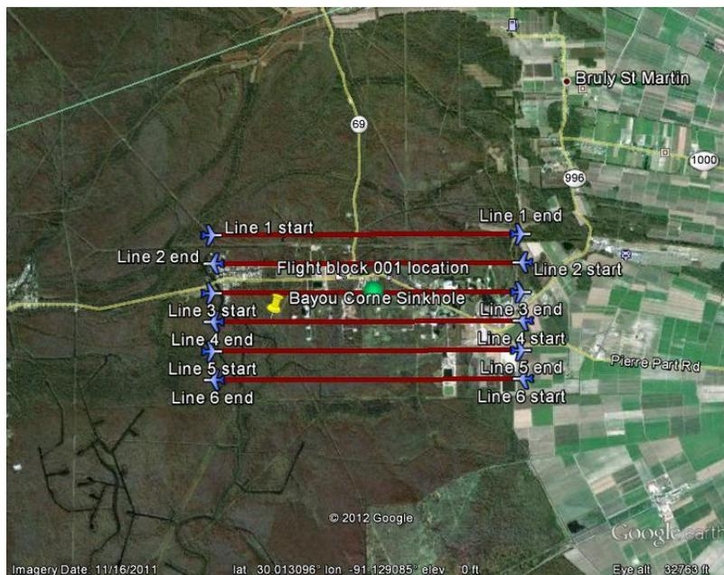
**Figure 5:** Flight planning lines for the chemical survey over Bayou Corne Sinkhole site
