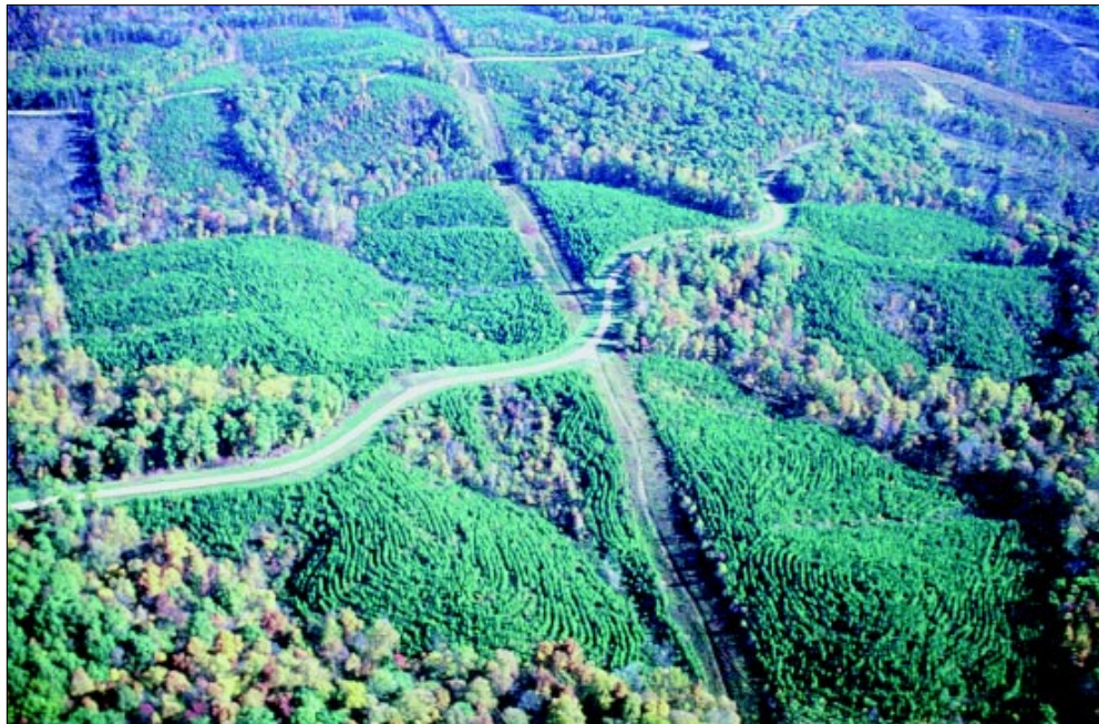
SMZs provide a water filtration strip of ground cover on ephemeral areas.
