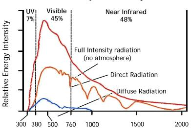
Figure 6-4 Relative Intensity of the Solar Spectrum
