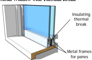
Figure 6-5 Metal Window with Thermal Break
