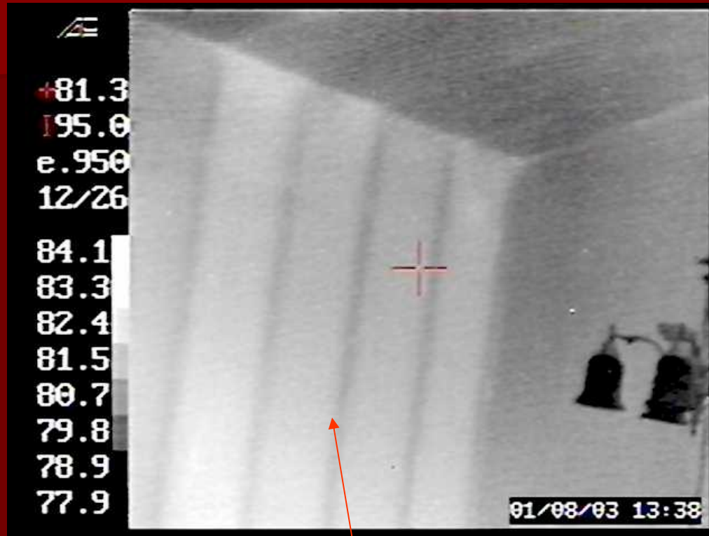
Chimney chase that is open to the attic and therefore a knee wall.
