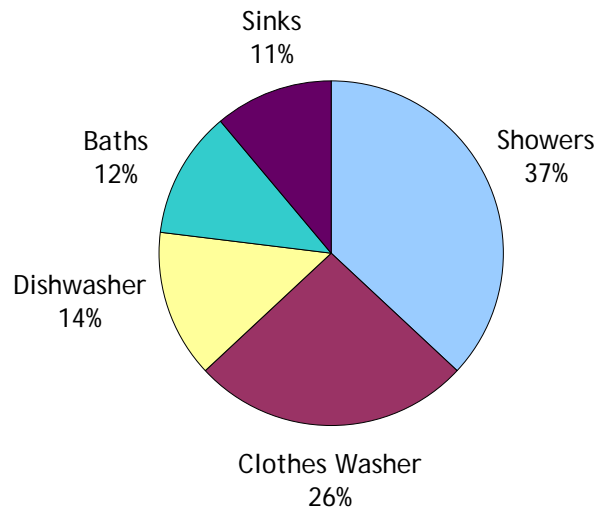
Figure 9-1 Typical Breakdown of Hot Water Use
